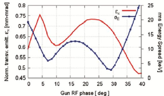
Figure 4: Gun RF phase scan. Normalized emittance and rms energy spread at 0.25m from photocathode.
