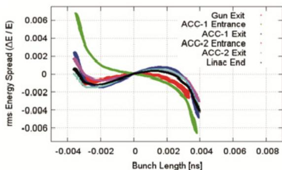
Figure 6: The longitudinal phase space profiles at the gun exit, entrance and exit of the first and the second accelerating sections.
