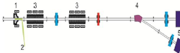
Figure 1: Schematic layout of AREAL 20 MeV S-Band linear accelerator. 1- RF –photo gun, 2- laser, 3- S-Band accel. sections, 4 –spectrometer, 5 - Beam dump.
