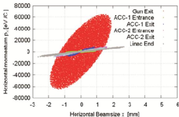
Figure 5: Transverse phase space profiles at the gun exit, entrance and exit of the first and the second accelerating sections.
