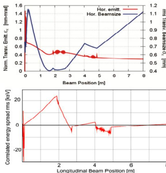
Figure 7: Transverse normalized emittance, beamsize (top) and correlated energy spread (bottom) evolution along the linac.
