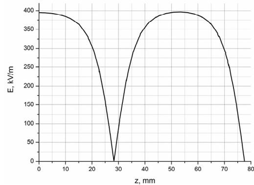
Figure 2: Accelerating field distribution along 1.6 cell structure axis.
