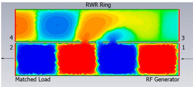
Figure 5: Directional coupler electrical field distribution.
