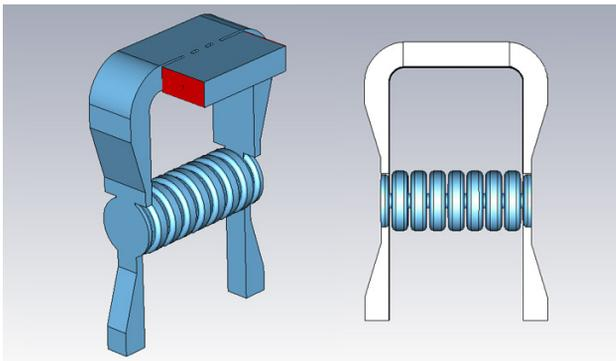
Figure 4: General view of TWR accelerating system.
