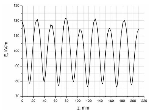
Figure 3: Accelerating field distribution along 7 cell and 2 half-cell structure axis.
