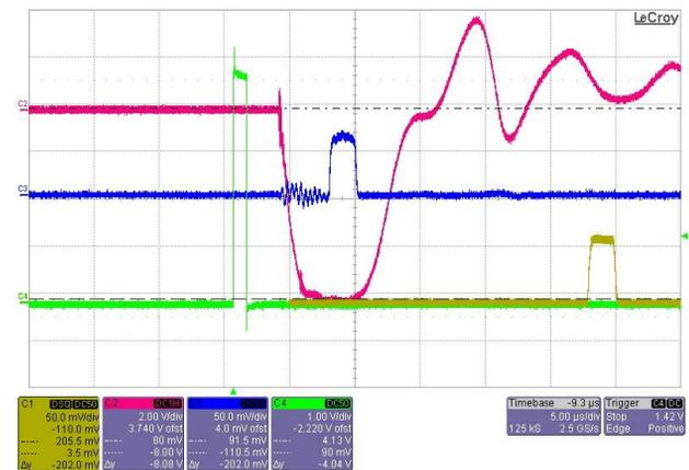
Figure 6: The klystron voltage signal (red) and the klystron output signal at saturation (blue).
