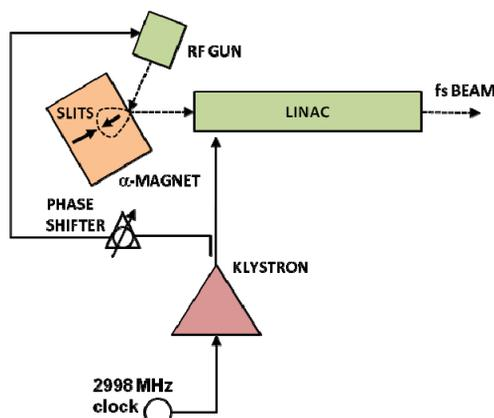
Figure 1: Schematics of the NSRRC low energy thermionic rf gun linac system for ultrashort beam generation with velocity bunching.
