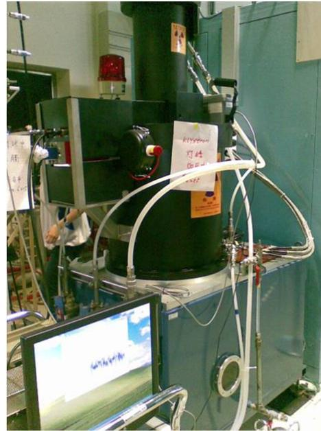
Figure 5: The 35 MW TH2100A klystron system.
