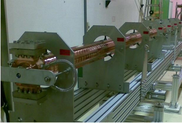
Figure 7: The S-band accelerating structure used in this setup.
