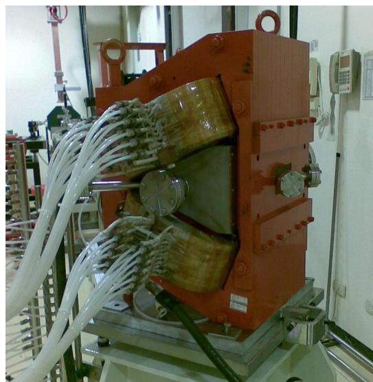
Figure 2: The alpha magnet with vacuum chamber.
