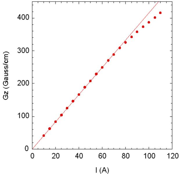
Figure 3: The measured relation of excitation current with magnetic gradient along the longitudinal direction.
