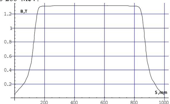
Figure 4 Longitudinal distribution of magnetic field along reference orbit ( $I_B=300$  A).
