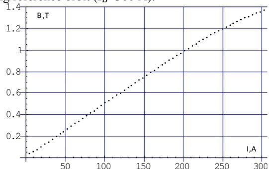
Figure 5: The magnetization curve of the first NESTOR storage ring bending magnet.
