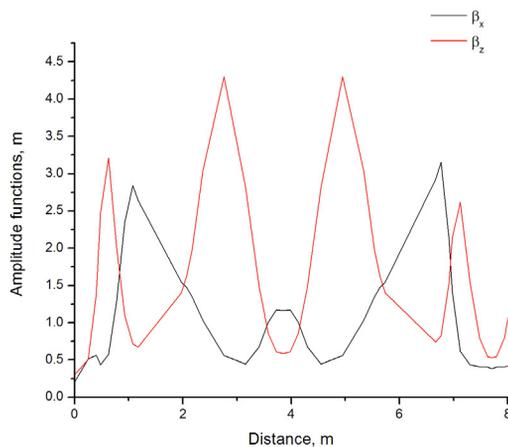
Figure 2: NESTOR X-ray source storage ring lattice beta functions.
