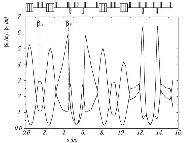
Figure 6: NESTOR X-ray source storage ring modified lattice beta functions.
