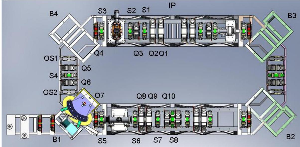
Figure 1: NESTOR X-ray source storage ring lattice layout. B1-B4 are dipole magnets with combined focusing function, Q1-Q10 are quadrupole magnets, S1-S7 are sextupole magnets, OS1-OS2 are octupole magnets combined with sextupole magnets.
