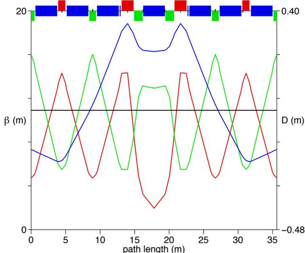
Figure 4: Newest basic block of the eRHIC arc where the elements are 2.6 times scaled up to reduce their overall number and improve on the packing factor. Dipole length is 3.12 m with a bending radius of  $\rho=234.2$  m.
