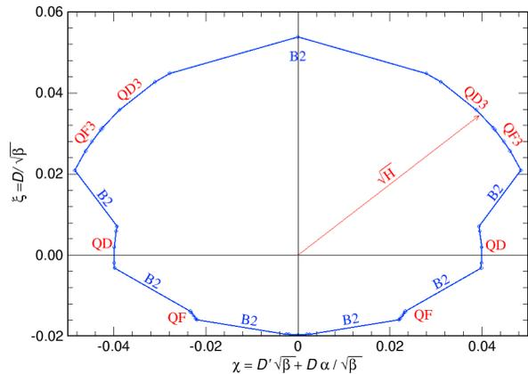
Figure 1: The normalized dispersion space for the basic module of the eRHIC arc. The B2 dipole vectors  $\chi = \theta \sqrt{\beta}$  shown are placed symmetrically with respect to the zero of the  $\xi$  axis making for the presented module the momentum compaction equal to zero ( $\alpha=0$ ).
