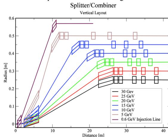
Figure 6: Splitter/Combiner define betatron functions in the linac for appropriate energies and provide connections to the arcs.
