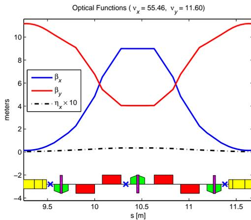
Figure 1: BPMs and correctors considered for TME arc cell. Steering correctors are shown in purple as additional windings on sextupoles, and BPMs indicated as blue crosses.
