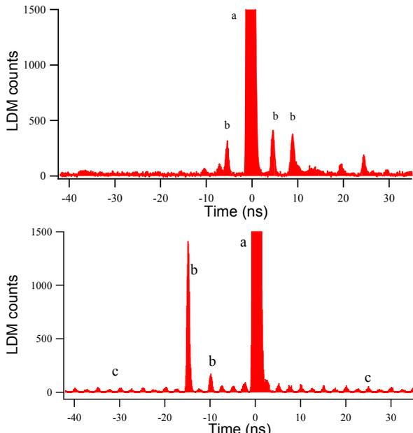
Figure 3: Typical pattern of satellites in an LHC fill with protons (above) and with lead ions (below) showing a) main bunch with peak at  $1.3 \times 10^5$  counts, b) satellites, and c) ghost bunches.
