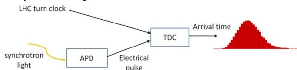
Figure 1: Schematic of the longitudinal density monitor.
