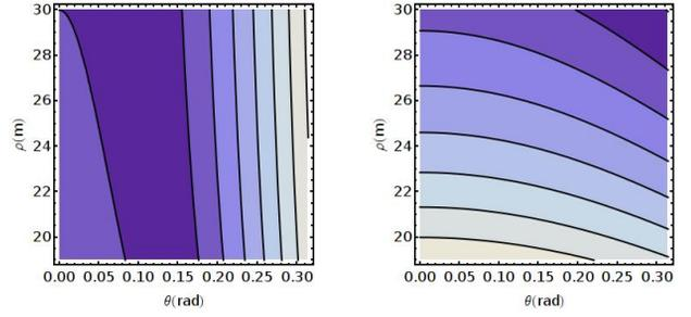
Figure 2:  $\alpha_0$  with respect to bending radius  $\rho_x$  and bending angle  $\theta$ , for  $\eta_c = -0.015m$  (left) and  $\eta_c = -0.8m$  (right). Darker areas represent smaller absolute values of  $\alpha_0$ .
