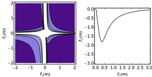
Figure 4:  $a_c$  of the TME cell with respect to  $f_1, f_2$  (left) and the curve for sets of values of  $f_1, f_2$  that are solutions for  $a_c = 0$  (right).
