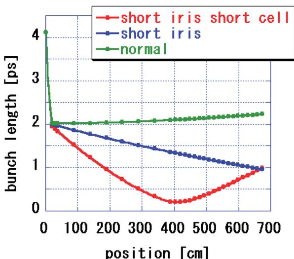
Figure 9: Bunch length as a function of distance from cathode.
