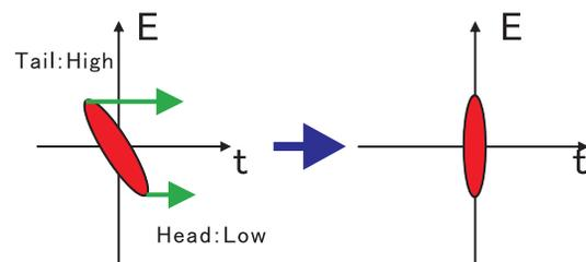
Figure 1: Principle of bunch compression.
