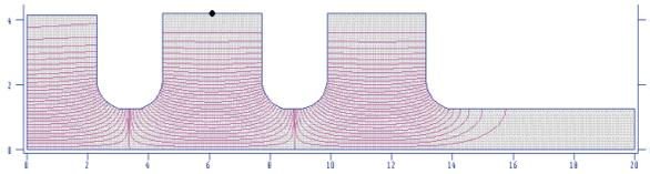
Figure 3: Structure of normal 2.6 cell RF-gun.
