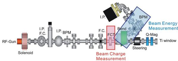
Figure 6: The Schematic design of Beamline
