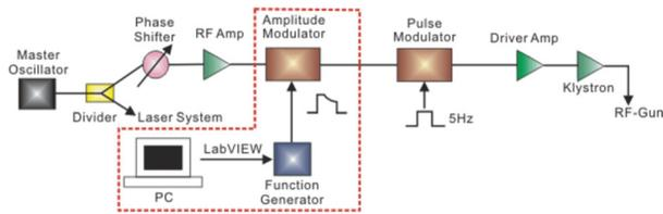
Figure 4: RF Control System for  $\Delta A$  Method
