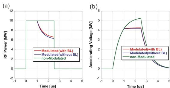
Figure 2: Calculations of (a)Input RF Pulse and (b)Accelerating Voltage
