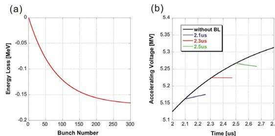
Figure 3: Calculations of (a)Beam Loading Loss and (b)Influence on the Accelerating Voltage
