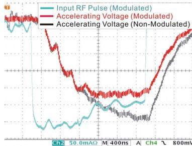
Figure 5: Observations of Input RF Pulse and Accelerating Voltage
