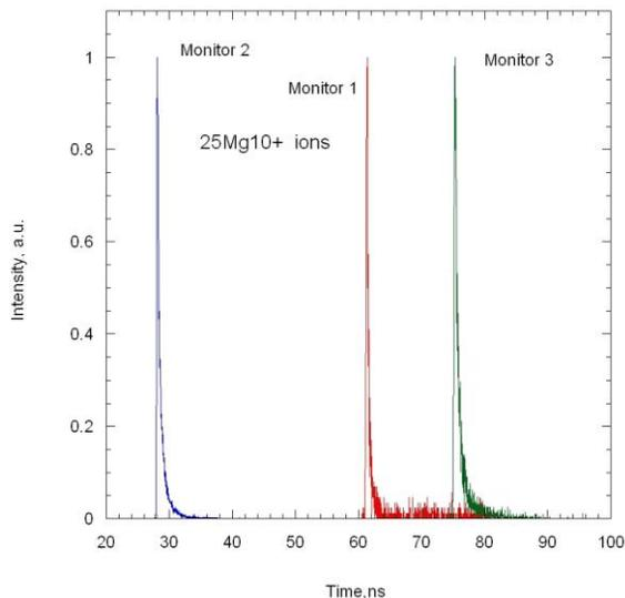
Figure 5:  $^{25}\text{Mg}^{10+}$  pilot ion beam time spectra. Each peak is normalized to its maximum.
