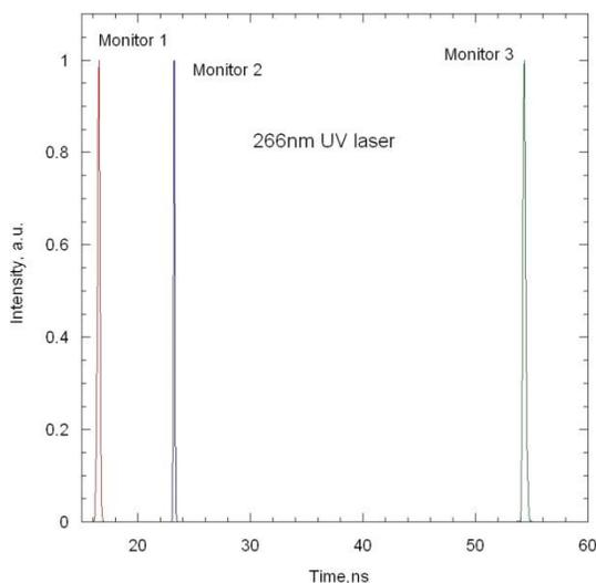
Figure 4: Calibration laser time spectra. Each peak is normalized to its maximum.
