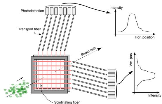
Figure 1: Schematic illustration of a detector for beam profile measurements based on scintillating optical fibers.
