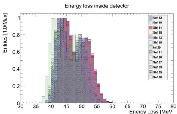
Figure 6: Energy loss of the fragments after traversing through gas volume and single Mylar structure.
