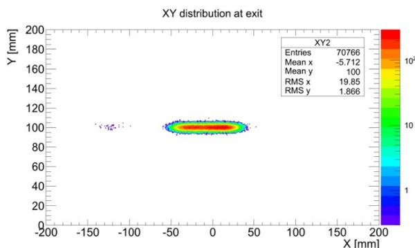
Figure 4: XY-distribution of fragments after flying through GEM-TPC gas volume of P10.
