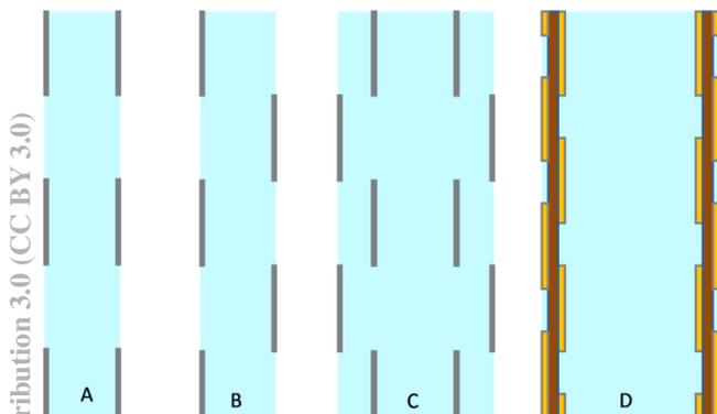
Figure 3: Different detector wall geometries used in the simulations. The dimensions of the elements are not in scale. A represents the configuration used in the prototype GEM-TPC, B with interlocked strips, C with double strips and D with strips etched on copper coated Kapton foil.
