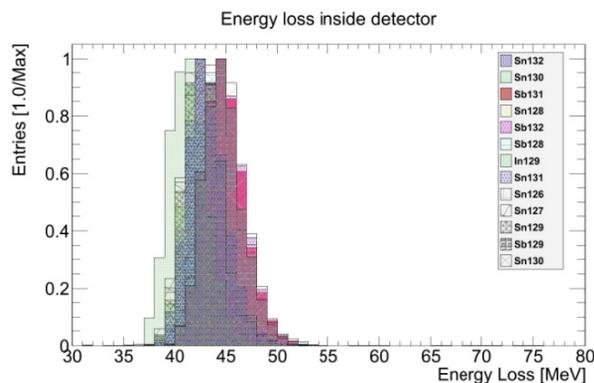
Figure 5: Energy loss inside gas volume of GEM-TPC.
