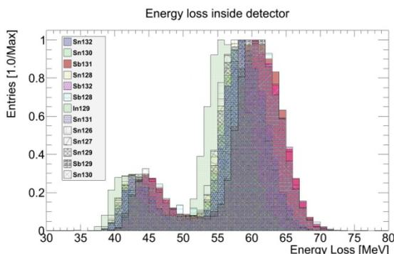
Figure 8: Energy loss of the fragments after traversing through gas volume and polyimide with copper strips.
