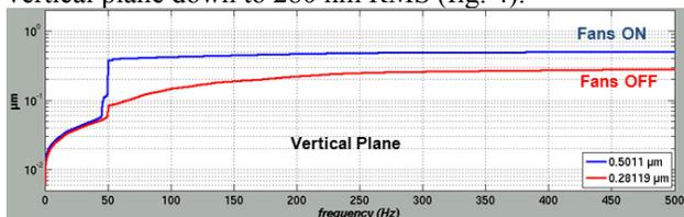
Figure 4: Integrated PSD (averaged over all BPMs) on the 0.1-500 Hz range in the vertical plane. With fans switched OFF (red curves) integrated noise is below 300 nm.
