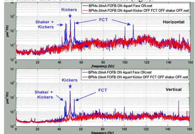
Figure 2: Beam orbit power spectral density (PSD) measurements (averaged over all BPMs) when fans are switched ON (blue curves) and OFF (red curves).
