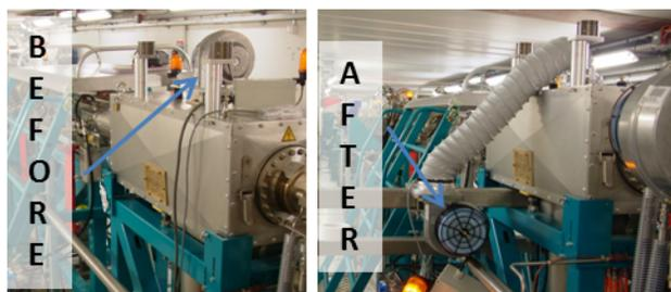
Figure 3: Kicker K2 fan at initial position (left) and with adjustable support (right).
