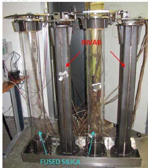
Figure 5: INVAR and fused Silica expansion measurement bench.
