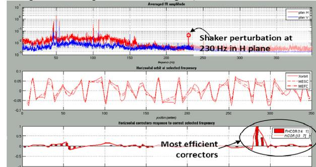
Figure 1: Diagnostic tool for noise source localization. An intentional excitation at 230 Hz is located.
