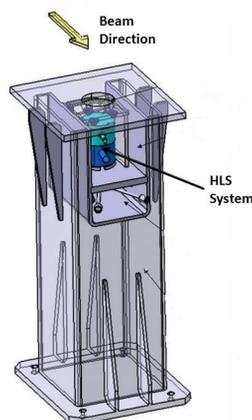
Figure 6: Drawing of the INVAR XBPM support for Nanoscopium. HLS sensor is hosted directly in the stand.
