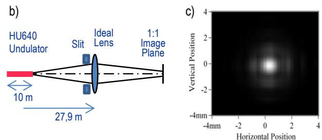
Figure 3: HU640 SRW calculation a) Undulator resonance energy (single-electron flux through pinhole) and experimental energy (multi-electron flux through finite aperture) b) Single-e radiation propagation scheme for coherence evaluation c) Intensity distribution in 1:1 image plane for the single-e radiation at the experimental energy.
