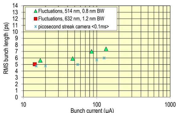
Figure 5: Bunch length measurements in low- $\alpha$  mode ( $\alpha_{nom}/10$ ) from HU640 radiation,  $V_{RF}=4$  MV.
