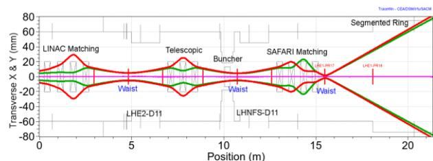
Figure 2: 5RMS deuterons beam envelopes along the LHE1 using TraceWin code [6].  $\phi_{BS}$  entrance=154mm.
