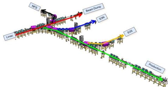
Figure 1: 3D view of the HEBT lines: LHE1 (red), LHE2 (green), LHNFS (black), LHS3N (blue).
