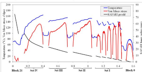
Figure 4: Temperature and Von Mises stress on SAFARI inner face using Ansys calculation.
