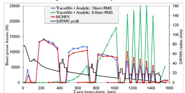
Figure 3: 40MeV-5mA deuterons beam power losses along SAFARI axis for a TraceWin/analytic calculation with  $RMS_{x,y}=16mm$  (blue),  $RMS_{x,y}=6.6mm$  (green) and MCNPX calculation (red).
