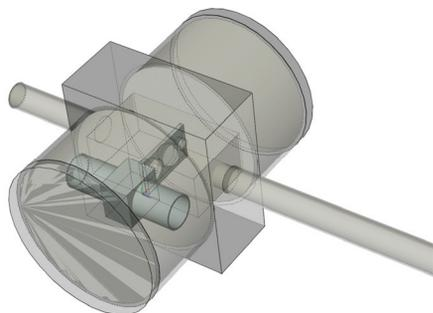
Figure 1: Model of the OTR screen. The external surfaces are made transparent to show the internal structure.
