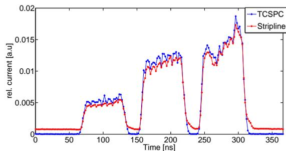
Figure 3: Multi bunch filling pattern recorded by TCSPC (blue curve) and a stripline (red curve).
