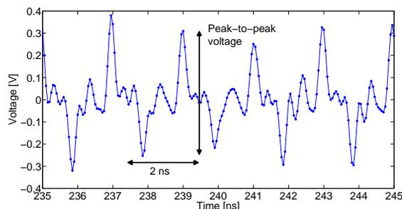
Figure 2: Detailed view of the stripline signal for a multi bunch filling-pattern. The signal consists of two pulses per bunch and the peak-to-peak voltage is taken as relevant value.
