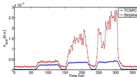
Figure 4: Standard deviation of a multi bunch filling pattern measured by TCSPC (blue curve) and a stripline (red curve).
