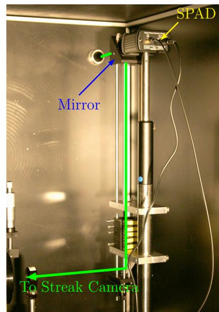
Figure 1: TCSPC-setup at the visible light diagnostics beamline, the setup is shielded by a metal box.
