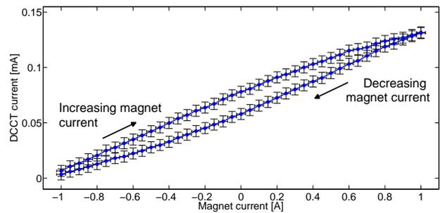
Figure 7: Current offset induced in the DCCT by the horizontal corrector magnet 3.1 installed close to the DCCT.
