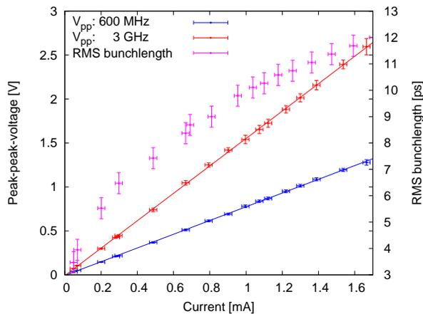
Figure 6: Decay of the stripline peak-to-peak voltage over bunch current, detected with oscilloscopes with different bandwidths (red and blue curve). The pink curve shows the bunch length decay over the current.
