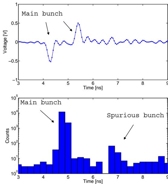
Figure 5: Stripline (above) and TCSPC (below) raw data for a single bunch fill.
