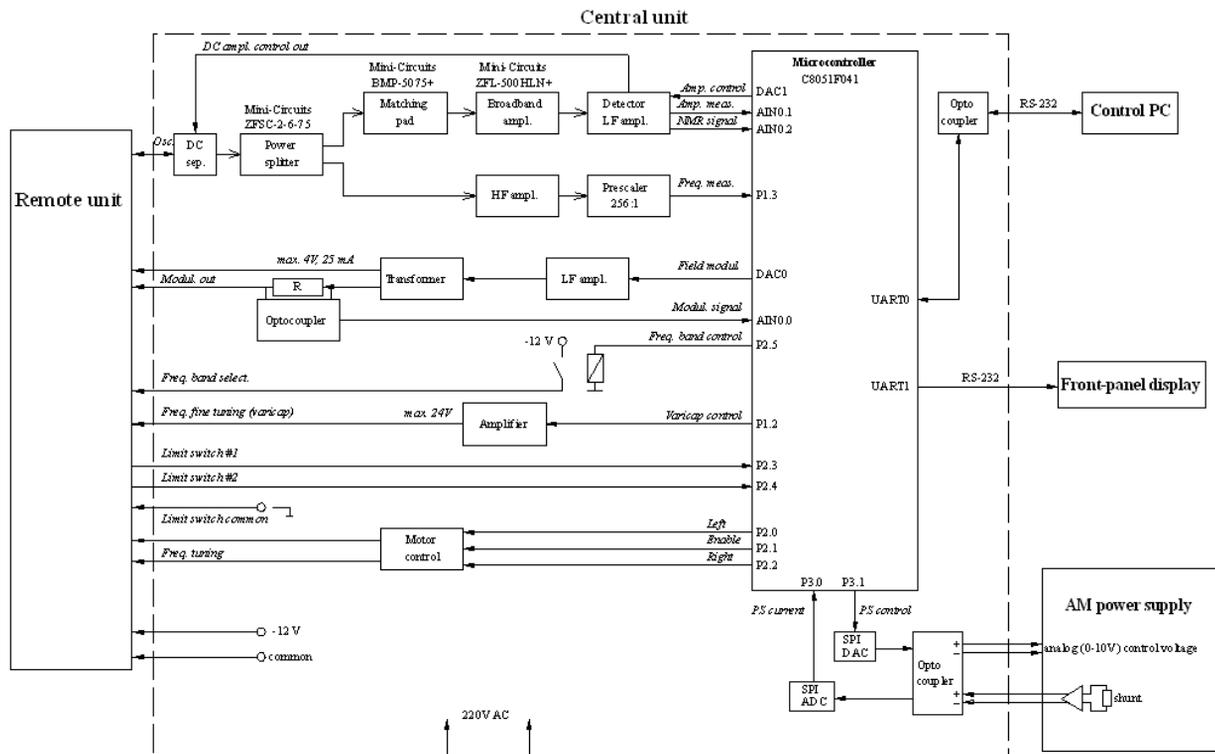
Figure 1: Block diagram of the new central unit with its connections to the rest of the system.
