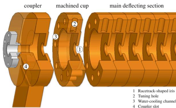
Figure 1: Schematic cut-off view of the C-band deflector, RAIDEN.
