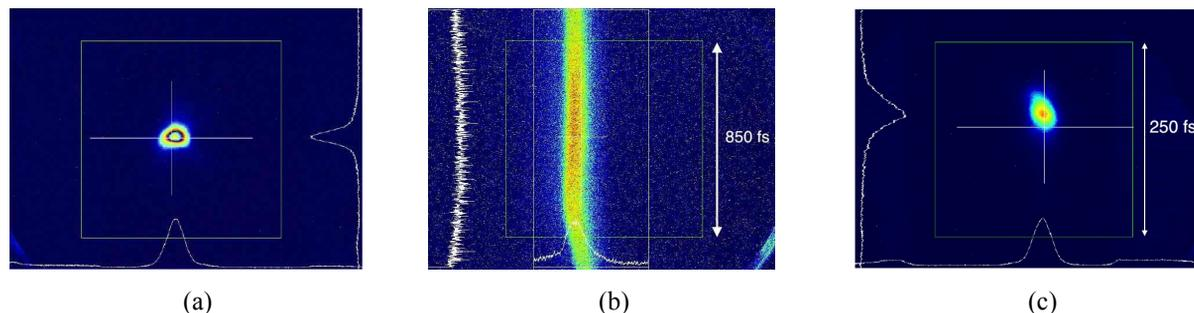
Figure 5: Bunch profiles on a Ce:YAG screen. (a) A bunch profile without deflection voltage; (b) the profile of a bunch of about 1 ps at  $V_T = 19$  MV; (c) the profile of a bunch of about 40 fs at  $V_T = 60$  MV.
