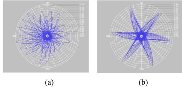
Figure 3: Phasors of deflecting fields within one of the RAIDENs by bead-perturbation measurement (a) before tuning and (b) after tuning.
