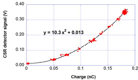
Figure 4: CSR intensity at the BC2 as the function of the beam charge.
