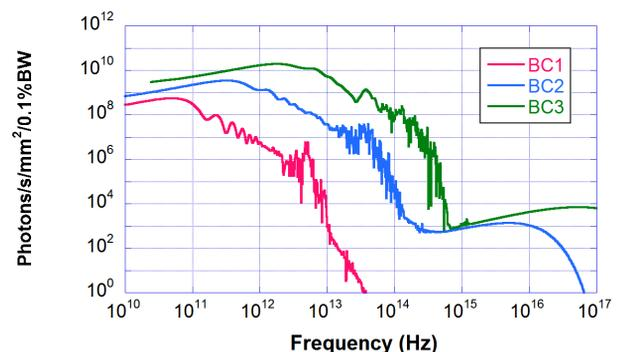
Figure 1: Calculated CSR spectrum at the BC sections by using SPECTRA [6].
