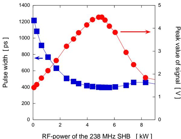
Figure 5: Output response of CT -476 versus RF-power of the 238 MHz SHB. One is the pulse duration (FWHM), and the other is the peak value of the output signal from the CT.
