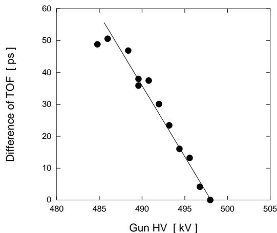
Figure 6: Difference of time-of-flight (TOF) measured by CTs in the injector part of the SACLA. TOF is plotted under the assuming that TOF is zero at gun HV of 498 kV.
