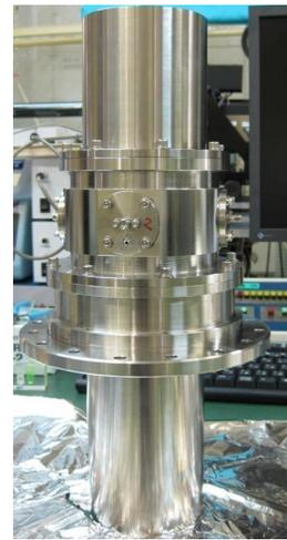
Figure 1: Cold model cavity BPM.
