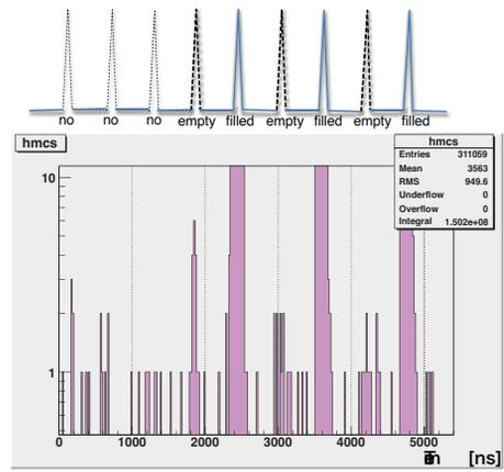
Figure 7: Timing distribution of secondary beam particles.
