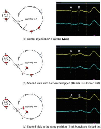
Figure 5: Residual beams with double injection kicking: (a) No double kicking, (b) with double kicking for the 2nd bucket and (c) with double-kicking for both buckets.
