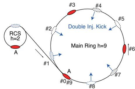
Figure 8: New scheme of MR Injection for COMET.
