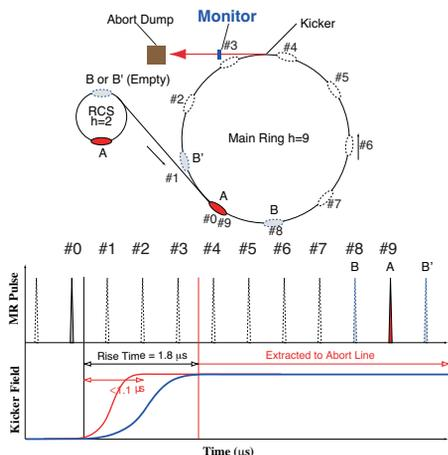
Figure 2: Beam diagnosis by using fast-extracted beam
