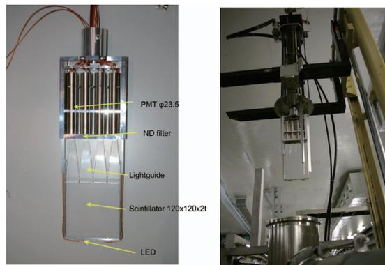
Figure 3: A New beam monitor used for the abort line measurements.
