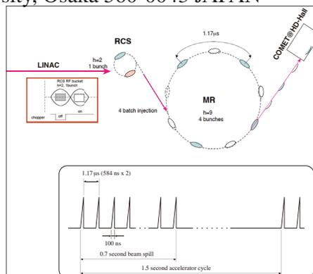
Figure 1: Simplest scheme of MR Injection for COMET experiment.
