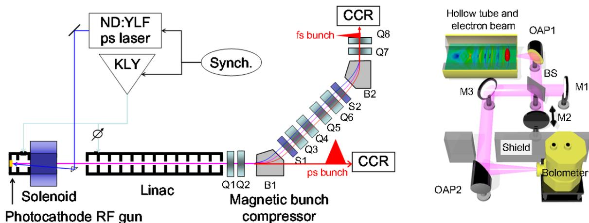
Figure 1: (Left) Photocathode RF gun linac with a magnetic bunch compressor of an achromatic arc. (Right) Diagram of multimode CCR and measurement system. OAP denotes an off-axis parabolic mirror; M, a plane mirror; BS, a beam splitter.
