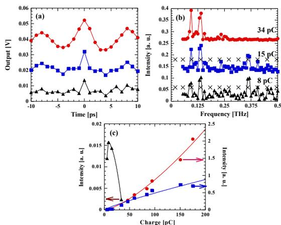
Figure 3: (a) Interferograms near the centerburst position for 34, 15 and 8 pC bunch charges with offsets and factors adjusted for comparison. (b) Frequency spectra for 34, 15 and 8 pC bunch charges with offsets and factors adjusted for comparison. The theoretical frequencies of  $TM_{0n}$  modes (cross) were shown. (c) Intensities for  $TM_{03}$ ,  $TM_{04}$  and  $TM_{09}$  modes as a function of the bunch charge.
