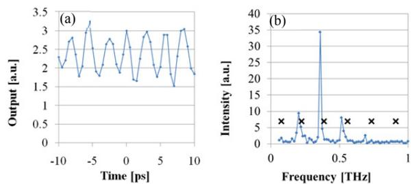
Figure 4: (a) Interferogram from a tube with inner radius/outer radius/ tube length of 1/1.5/150 mm. (b) Frequency spectrum for the other tube. The theoretical frequencies of  $TM_{0n}$  modes (cross) were shown.
