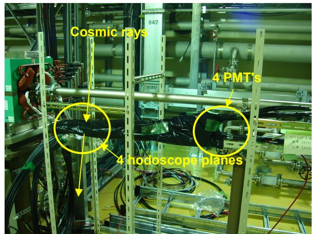
Figure 4: A setup for cosmic ray measurements.
