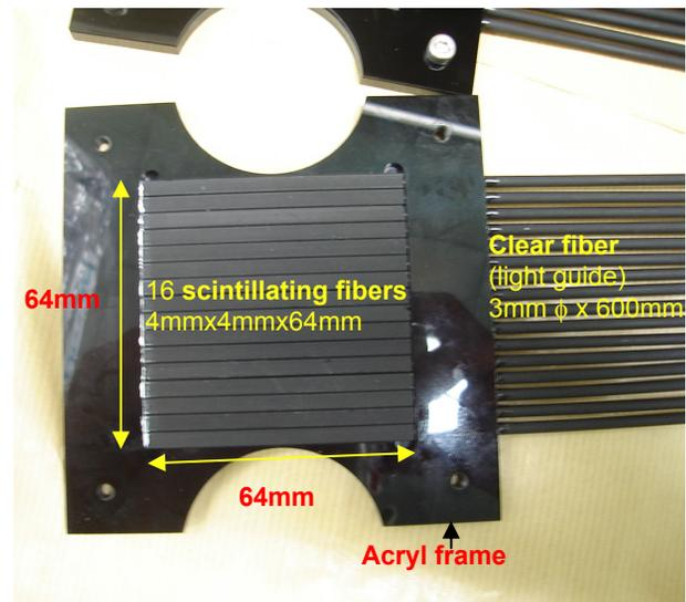
Figure 1: A scintillating fiber hodoscope.
