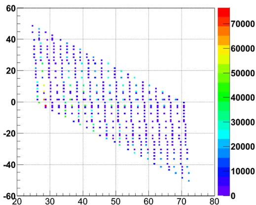
Figure 6: Horizontal positions at H0 (x-axis) (mm) (the origin is at the beam axis) and track angles with respect to the beam axis (mrad) for tracks with hits in all 4 hodoscope planes.
