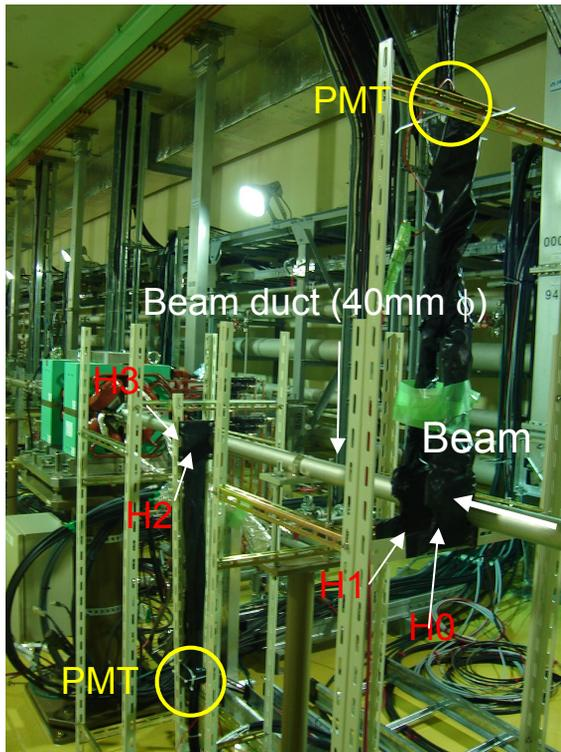
Figure 2: Experimental setup of beam loss measurements in the ACS section.
