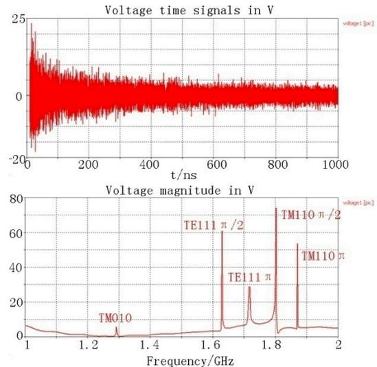
Figure 4: The simulation results of the HOMs excited by a single bunch.
