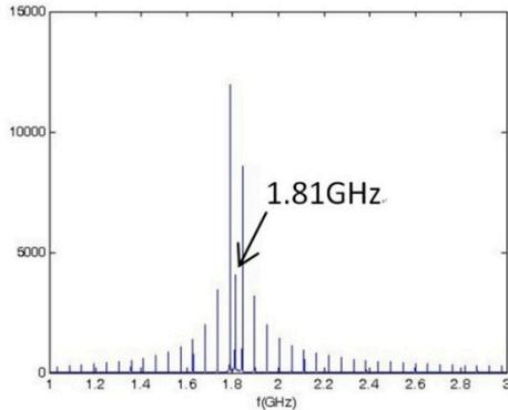
Figure 2: The spectrum of one mode voltage caused by high repetition beam.
