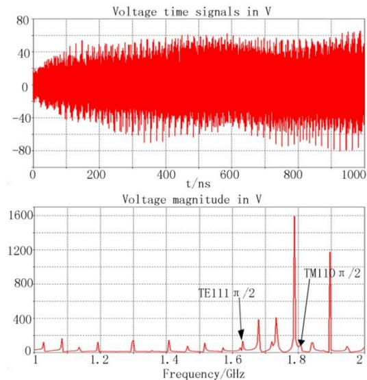
Figure 5: The simulation results of the HOMs excited by high repetition bunches.
