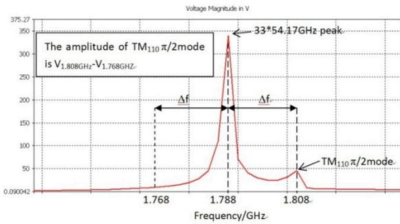
Figure 6: The HOMs amplitudes are found with both kinds of peaks.
