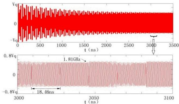
Figure 1: The waveform of one mode voltage caused by high repetition beam.
