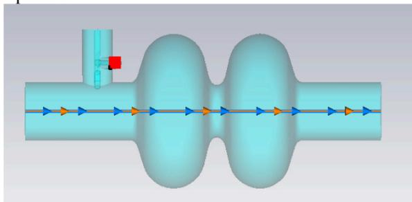
Figure 3: The TESLA 2-cell cavity model used for simulation.
