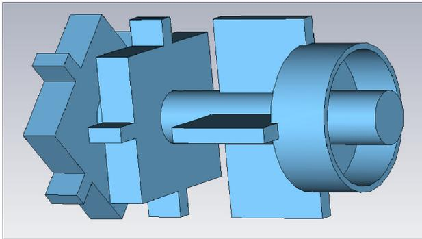
Figure 5: Multi-cell cavity beam monitor
