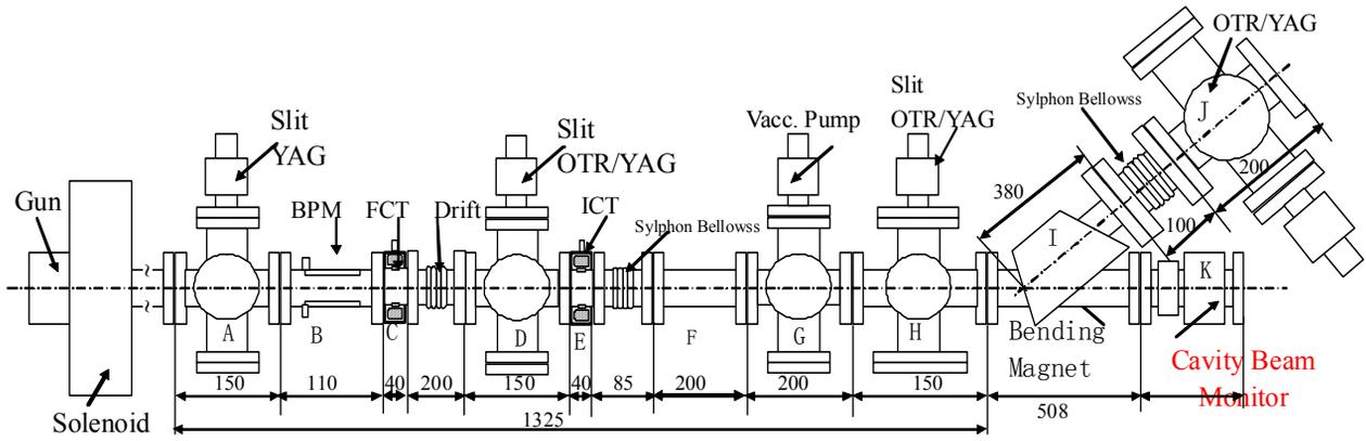
Figure 2: Complex installation drawing of beam diagnostic system
