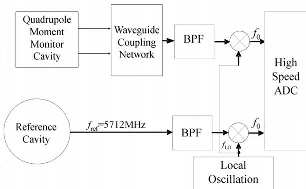
Figure 6: Signal processing system of beam quadrupole moment monitor
