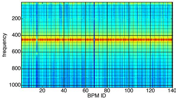
Figure 2: Horizontal position spectra of all BPMs. It shows BPM #15 and #68 different.
