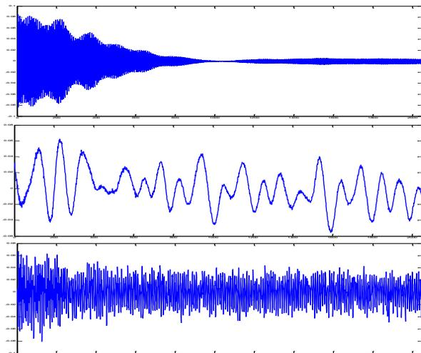
Figure 3: Betatron oscillation mode (top), energy oscillation mode (middle) and 68 kHz global electronics noise mode (bottom) retrieved from BPM TBT matrix using MIA method.
