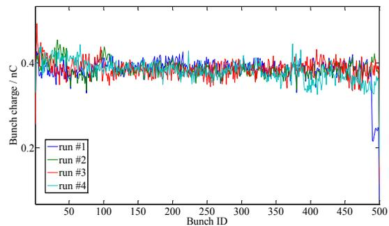
Figure 5: Repeatability of filling pattern recorded by current analyzer.
