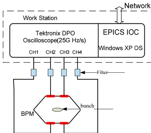
Figure 3: The schematic drawing of the system
