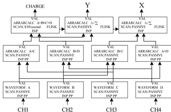
Figure 4: IOC software structure block diagram.
