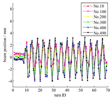
Figure 6: Position of 6 picked bunches in horizontal direction
