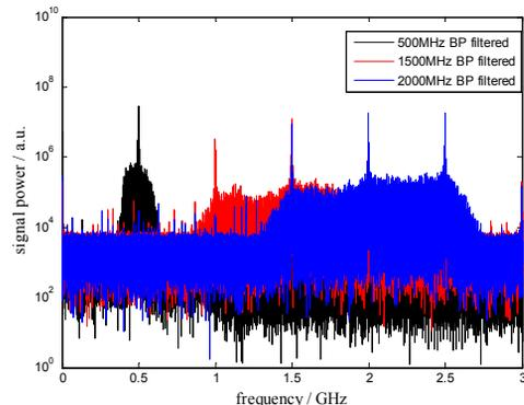
Figure 5: Signal power filtered by 3 types of filter.
