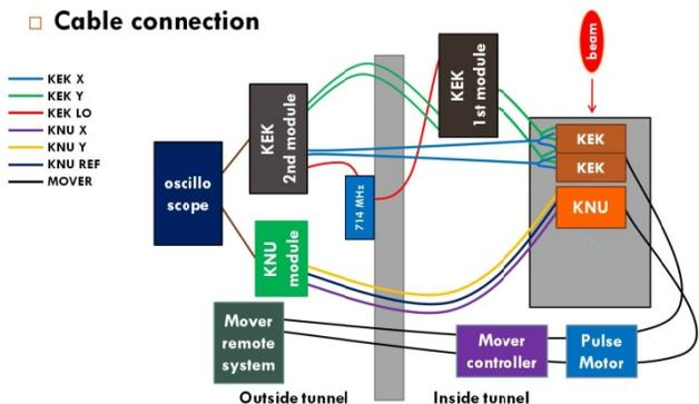
Figure 2: Beam position resolution measurement test scheme for Low-Q IP-BPM.
