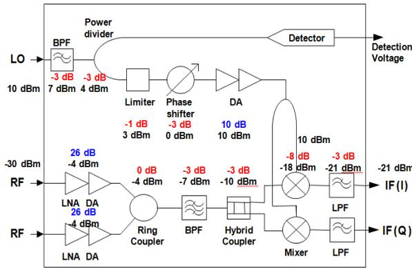
Figure 3: Electronics block diagram of Low-Q IP-BPM.
