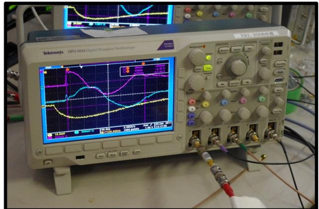
Figure 5: A one of the examples of I-Q tuning. The violet line shows I signal and sky-blue line shows Q signal.
