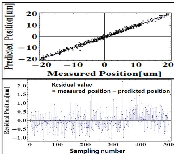
Figure 8: The measured position vs. predicted position (Top). Residual position due to 500 events (Bottom).
