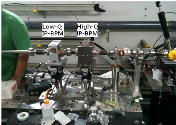
Figure 4: Installed appearance of Low-Q IP-BPM (Left) and High-Q IP-BPMs (Right).
