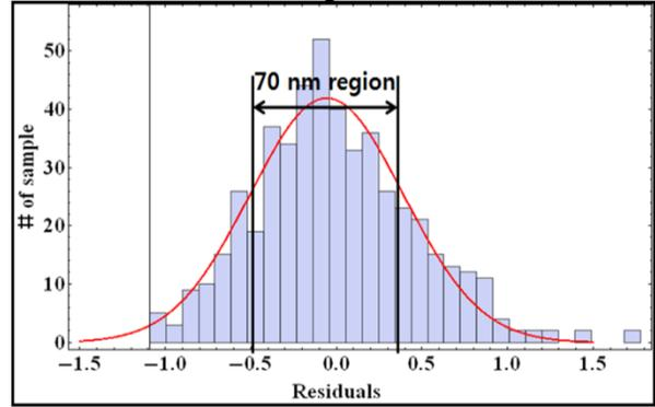
Figure 9: Gaussian fitting of residual position.
