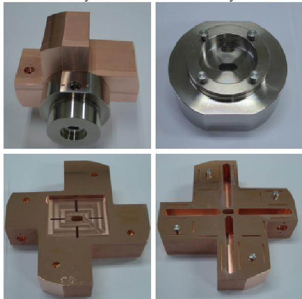
Figure 1: Entire of Low-Q IP-BPM (left up). Reference cavity (right up). Sensor cavity part (left down). Wave guide part (right down).
