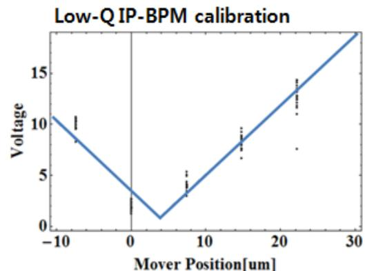
Figure 6: Low-Q IP-BPM calibration run under 40dB amplification condition.
