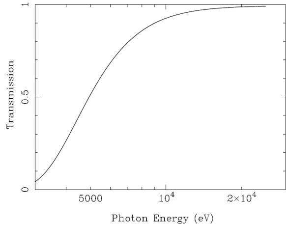
Figure 4: Dependence of the photon transmission through a diamond plate 100  $\mu\text{m}$  thick on the photon energy.
