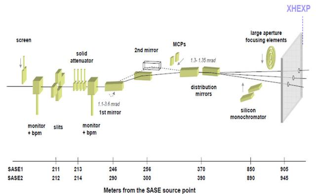
Figure 1: Schematic view of the SASE1&SASE2 mirrors and attenuators for the MCP.
