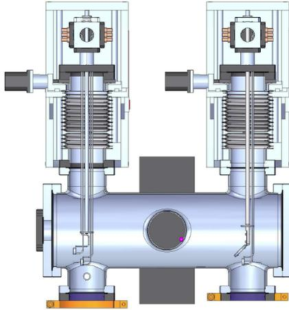
Figure 2: View of MCP detector for SASE1 and SASE2.
