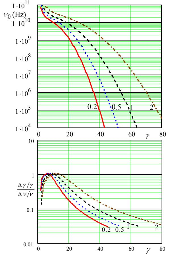
Figure 2: The mode frequency (top) and the ratio between relative accuracies of  $\gamma$  and frequency (bottom) depending on  $\gamma$ ;  $a = 3$  cm,  $r_0 = 0.5$  mm,  $d_z = 2\pi a/38 \approx 5$  mm; magnitudes of  $d_\phi$  (cm) are given close to the curves.
