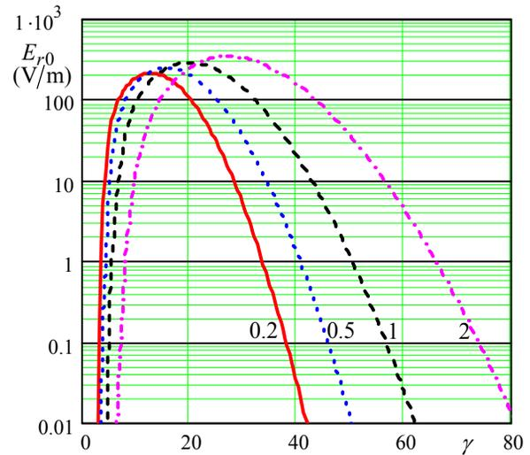
Figure 4: Amplitude of the component  $E_r^W$  on the outward surface of waveguide ( $r=a+0$ ) depending on  $\gamma$ ; magnitudes of  $d_\phi$  (cm) are indicated near the curves, other parameters are the same as in Fig 3.
