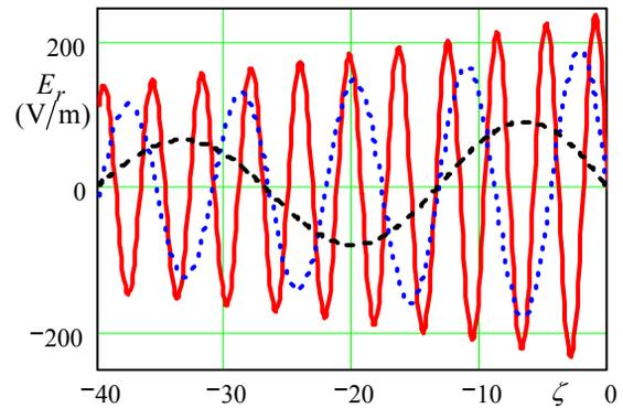
Figure 5: Component  $E_r^W$  on the outward surface of waveguide depending on the distance  $\zeta = z - Vt$  for  $\gamma = 15$  (solid red),  $\gamma = 20$  (dotted blue),  $\gamma = 25$  (dashed black). Conductivity of wires is  $5 \cdot 10^7 (\text{om})^{-1}$  (copper), other parameters are the same as in Fig 3.
