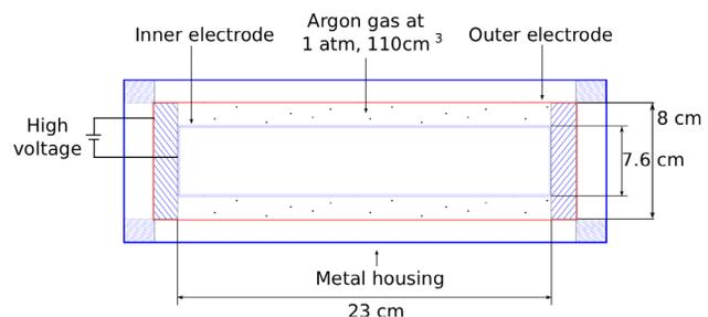
Figure 3: ESS prototype ionization chamber.
