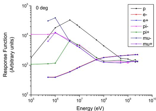
Figure 4: ESS prototype ionization chamber response function as a function of incident particle type and energy. For zero incident angle.
