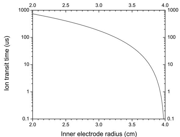
Figure 2: Cylindrical ionization chamber ion collection time as a function of the inner cylinder radius. The detector is filled with Argon gas at 1 atm pressure. Outer electrode radius is 4 cm, bias voltage - 3 kV and effective volume -  $110 \text{ cm}^3$ .
