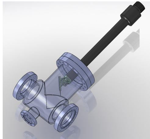
Figure 3: The vacuum chamber for the screen. The screen will be visible to the camera via a view-port at  $45^\circ$  angle.
