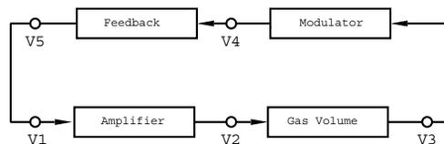
Figure 6: The conceptual setup of the ring oscillator. The gas volume in the ACS that we intend to probe is shown at the lower right.
