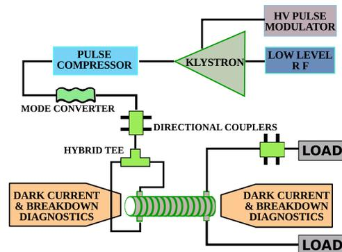
Figure 1: The klystron will deliver a peak RF power of 50 MW at 11.9942 GHz. The RF pulse is compressed and amplitude- and phase-modulated by the low level RF system. The RF power is transferred to the accelerating structure test area for conditioning and diagnostics.
