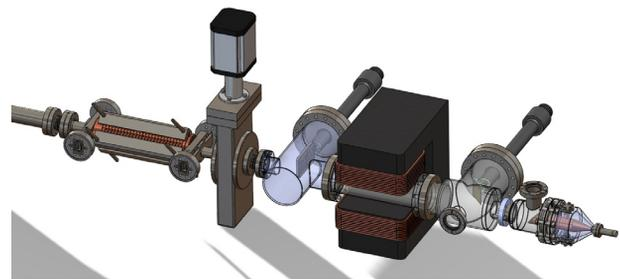
Figure 4: 3D-model of the diagnostic setup. Shown from the left are: the ACS followed by the vacuum valve connected to the chamber hosting pepper-pot grids, dipole magnet and fluorescent screen chamber with the view-port for the camera. The setup will be terminated by the Faraday cup equipped with a view-port.
