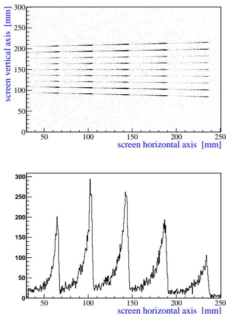
Figure 5: Pepper-pot pattern expected on the screen after the simulation of  $4 \times 10^6$  electrons generated with flat energy distribution 0.5-20 MeV with 5 mm-thick tungsten pepper-pot and magnet strength of 5 mT. Top: 2D picture, bottom: projection on the horizontal axis.
