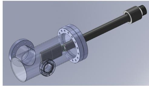
Figure 2: The vacuum chamber with 2 pepper-pot grids mounted on a linear manipulator. The grids can be fully extracted from the particle pathway.
