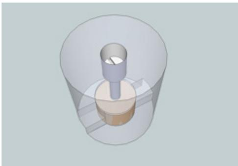
Figure 4: Capacitively coupled phase trimmer.
