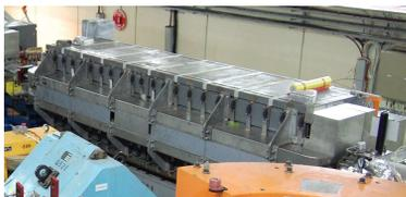
Figure 1: PS main magnet with a LHC-type BLM (yellow cylinder on top of the magnet) and an ACEM (orange cylinder in front of the magnet).
