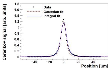
Figure 3: Vertical laser-wire scans in the ATF.
