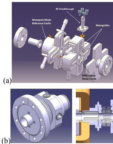
Figure 2: (a) Main Beam Linac Cavity BPM (b) 3D model of a Drive Beam Decelerator BPM and its integration in the CLIC module
