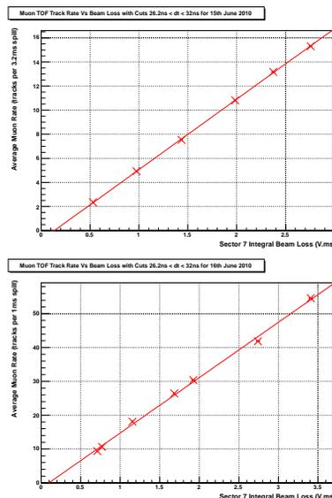
Figure 7: Average muon TOF track rate per spill as a function of induced ISIS beam loss for a negative  $\pi \rightarrow \mu$  beam, with a 3.2 ms spill gate (top), and for a positive  $\pi \rightarrow \mu$  beam, with a 1 ms spill gate (bottom).
