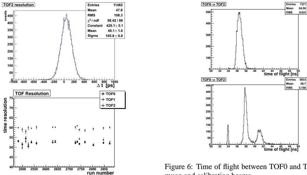
Figure 6: Time of flight between TOF0 and TOF2 for the muon and calibration beams.
