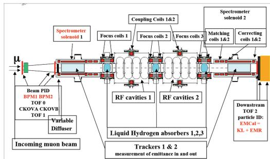
Figure 1: View of the MICE experiment at RAL. The muon beam from ISIS enters from the left. The cooling channel is put between two magnetic spectrometers and two TOF stations (TOF1 and TOF2) to measure particle parameters.
