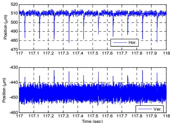
Figure 8: Orbit excursion due to septum & kicker field leakage during injection.
