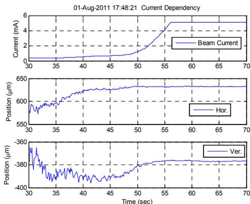
Figure 5: SA data for real beam. Current from 0 mA to 5 mA. Input power level of the Libera Brilliance+ is set at -30 dBm.
