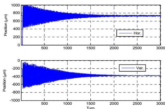
Figure 9: Turn by turn data. Betatron oscillation excited by injection.
