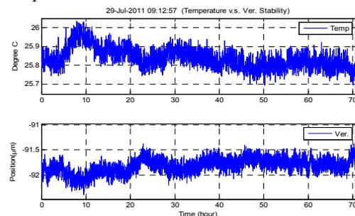
Figure 4: Temperature dependency test. The test site temperature is controlled within 0.2  $^{\circ}\text{C}$  during 72 hours.
