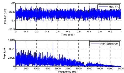
Figure 3: Horizontal FA data of time series and spectrum. There is a notch frequency near 3.3 kHz to compensate channel switch noise.
