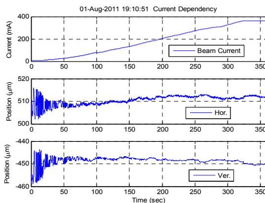
Figure 6: SA data for real beam. Current from 5 mA to 360 mA. Input power level of the Libera Brilliance+ is set at 0 dBm.
