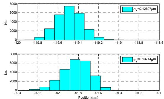
Figure 2: Histogram during 3 days at 0.1 Hz stability test.
