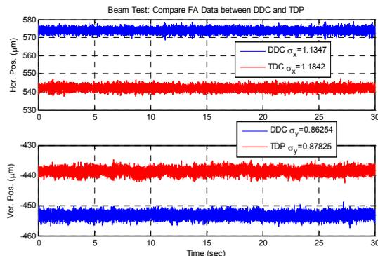
Figure 10: DDC and TDP FA data comparison of horizontal and vertical position for beam test.  $K_x$  and  $K_y$  are both set 10mm. Horizontal RMS of TDP 1.18  $\mu\text{m}$  is a little higher than DDC RMS 1.13  $\mu\text{m}$ . Vertical RMS 0.89  $\mu\text{m}$  of TDP is also higher than DDC RMS 0.86  $\mu\text{m}$ . The cause could be inferred from turn by turn data where TDP data with higher amplitude variation.
