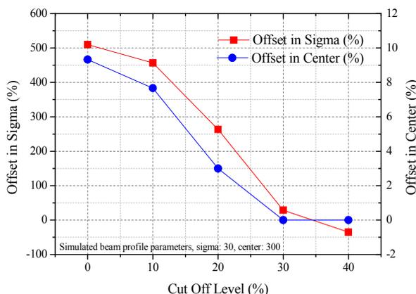
Figure 1: Cutting Level Affects under Nonzero-Mean Background Noise (10%) for Moment Method.
