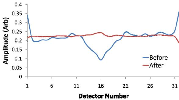
Figure 4: A comparison of IPM output before and after calibration of the MCP.
