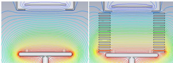
Figure 2: Simulations of transverse bias field at the centre of the IPM without (left) and with (right) the field shaping electrodes
