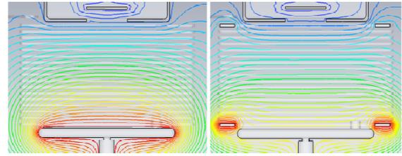
Figure 6: Longitudinal field within the IPM field shaping electrodes, without (left) and with (right) the longitudinal field corrector electrodes
