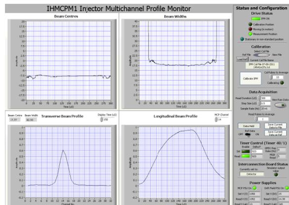
Figure 3: LabVIEW front panel of the IPM program
