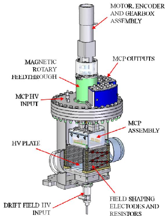
Figure 1: CAD drawing of the IPM assembly
