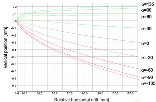
Figure 3: OPERA particle tracking simulations. The different tracks correspond to the trajectories of ions with different initial momentum direction, as described by the angle  $\alpha$  formed with the horizontal.  $\alpha = \pm 135^\circ$  corresponds to the outermost tracks (maximum ballistic range from trivial kinematic considerations), hence their distance at the detector level ( $z = 150$ ) expresses the resolution of the monitor: about 1 mm.
