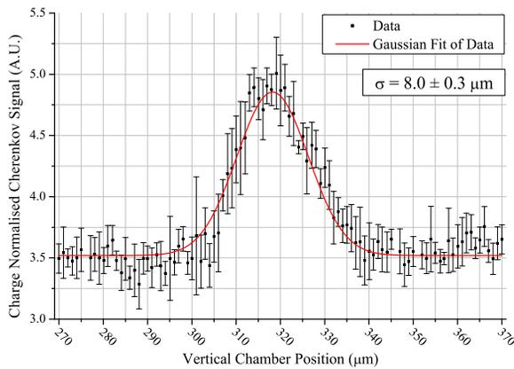
Figure 5: Vertical scan of tuned electron beam.
