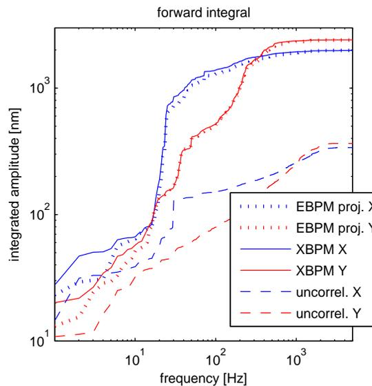
Figure 2: Integrated motion amplitudes of projected EBPM and XBPM positions (at the location of the XBPM), and uncorrelated components.
