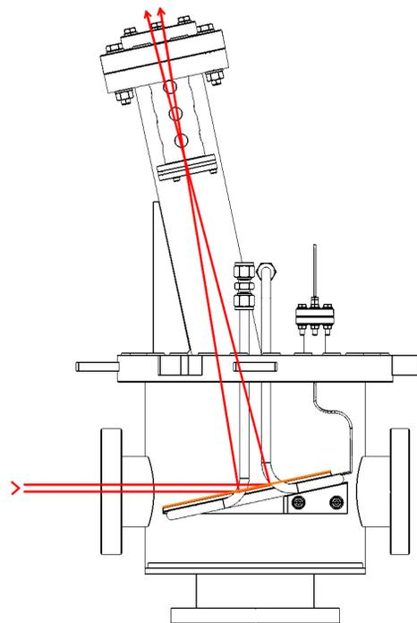
Figure 3: Cut view of the aperture XBPM: The red lines depict the path of X-rays in the outer region of the incoming beam, which are scattered by the surface of the copper aperture
