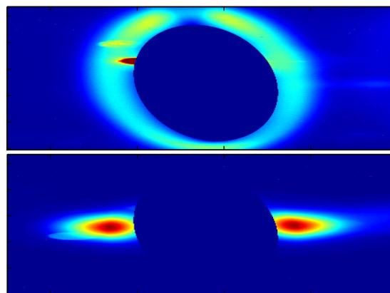
Figure 4: Example images of scattered photons for two different polarisations of the EPU: circular polarisation (top) and horizontal linear polarisation (bottom). Camera images have been processed to remove some artifacts from the area inside the aperture and to remove some of the distortion caused by the imaging geometry.
