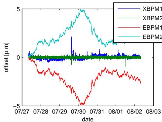
Figure 1: A 6 day record of vertical beam position offsets at two frontend XBPMs and 'golden orbit' offsets set by the slow feedback to keep the beam stable at XBPM2.
