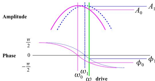
Figure 2: Steady state amplitude and phase response as the cavity resonant frequency changes from  $\omega_0$  to  $\omega_1$ .
