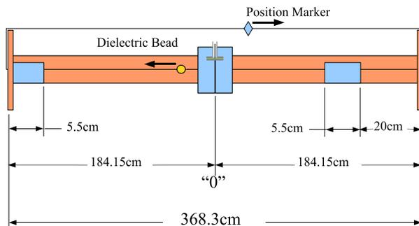
Figure 4: For bead pull measurements, a thin monofilament line varies the position of a dielectric bead in WR284 waveguide. The center flange has BPM-like buttons that are used to couple microwaves in/out of the waveguide.
