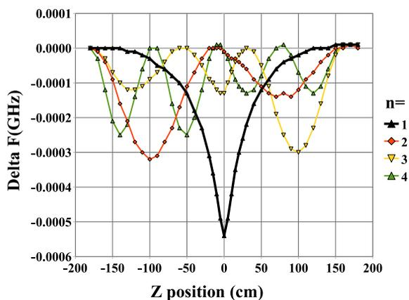
Figure 5: The cutoff resonance was observed using a modified drive flange in a measurement with WR284 waveguide.
