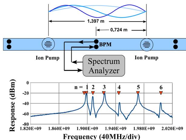
Figure 1: Sketch of 43E at CesrTA, where a BPM Detector is located between two ion pumps with longitudinal slots. The measured resonances follow the expected  $f^2 = f_c^2 + \left(\frac{nc}{2L}\right)^2$  of a rectangular cavity.
