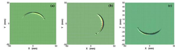
Figure 3: Dependence of screen image on the phase between the laser and electron bunch:  $0^\circ$ (left),  $90^\circ$ (middle) and  $180^\circ$  (right).
