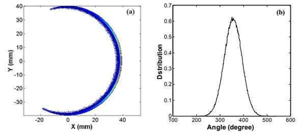
Figure 2: Image on the screen and its angular distribution, with laser field only.
