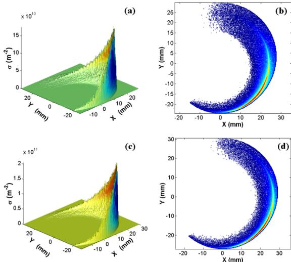
Figure 5: Particle area density (left) and image (right) on the screen with different beam size and laser power. (Top) the rms beam size is 10  $\mu\text{m}$  and the laser power is 1.8GW; (Bottom) The rms beam size is 15  $\mu\text{m}$  and the laser power is 5.0GW.
