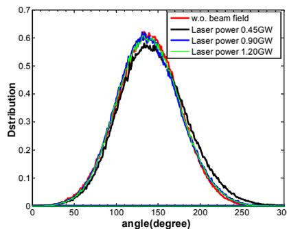
Figure 6: Effect of laser power on the angular distribution of the particles on the screen.
