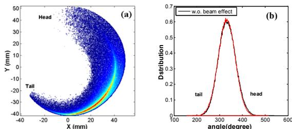
Figure 4: Image on the screen and its angular distribution with both beam field and laser field. The laser power is 1.2GW with a waist of 30mm.
