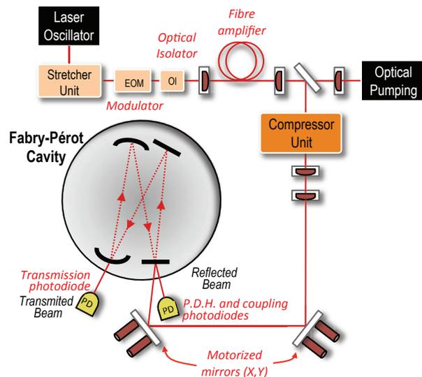
Figure 1: Optical layout of the experiment.
