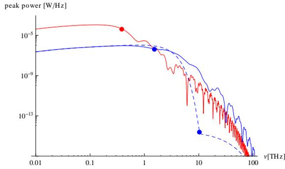
Figure 5: Power spectrum of the 3 nC (red) and 100 pC (blue) bunch. The points mark the power at frequencies corresponding to the bunch lengths (0.4 THz and 1.5 THz). The dashed curve depicts the spectrum of the Gaussian approximation of the 100 pC bunch with  $\sigma = 10$  THz.
