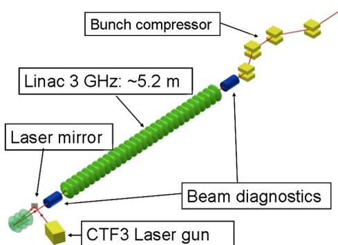
Figure 1: The concept of FLUTE with a 2 1/2 cell RF photo-gun and 3 GHz linear accelerator followed by a bunch compressor. The total length of FLUTE is about 12 m.
