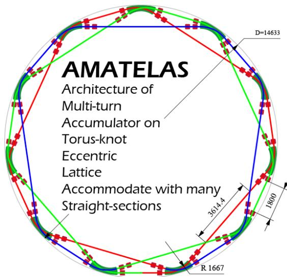
Figure 1: Schematic draw of (11, 3) AMATELAS designed for HiSOR-II.
