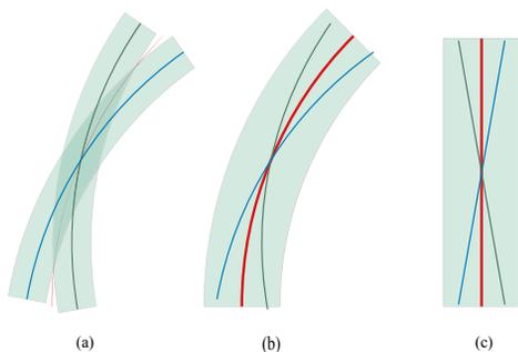
Figure 2: Crossed orbit in the bending magnet with gradient field.
