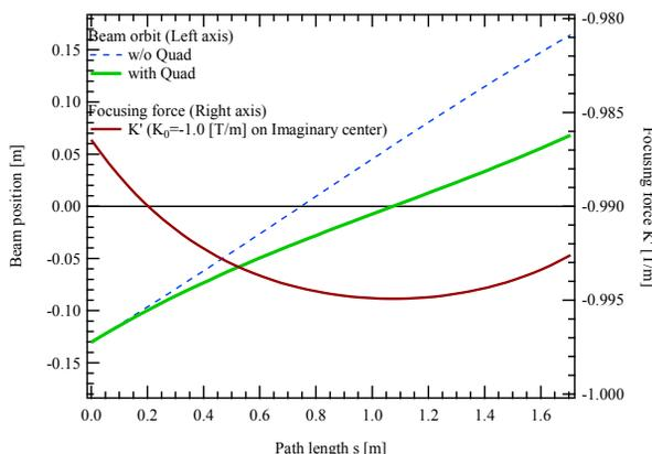
Figure 4: The deviation of focusing force along the orbit in the combined bending magnet.
