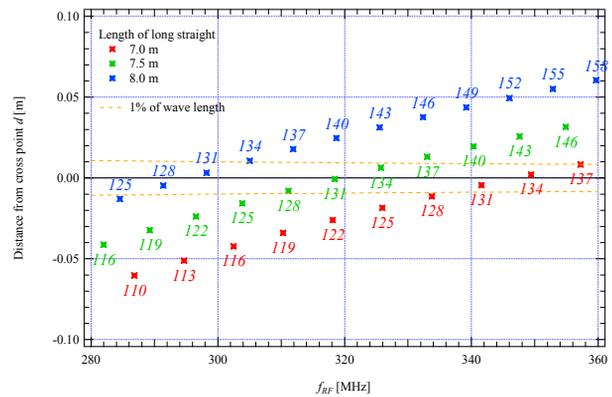
Figure 6: RF frequency and the harmonic number of conditions that the beams collide with each other.
